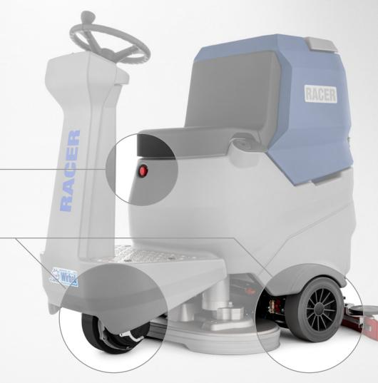
Automatic speed reduction on cornering at too high speeds.
