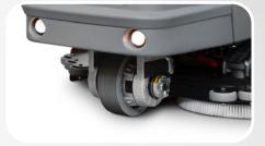
The new 900 W driving wheel guarantees RUNNER the best performance in terms of traction, resistance and high grade-ability. The front and rear non-slip and non-marking wheels ensure perfect stability, good grip and no slippery effects.
