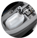
Chemical mixing system
